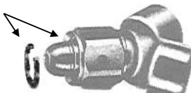
Part No. R-1 is a replacement ring for use with Item No's. 101, 102, 111 and 112. Slip ring in groove with nut in place and crimp closed.
