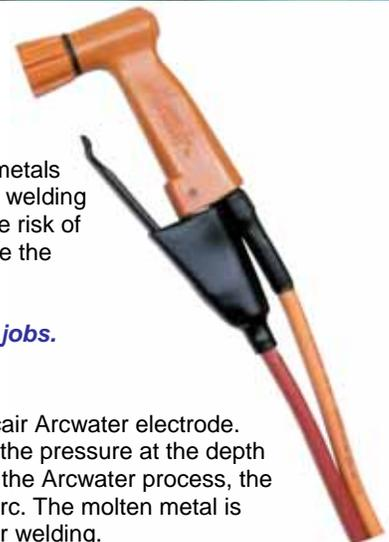
The Arcair® Arcwater® Torch is designed to gouge or cut steel, stainless steel and other metals underwater safely, easily and efficiently. Arcwater can also be converted to an underwater welding torch by simply changing collets. The unique Arcwater torch is **oxygen free**, eliminating the risk of hydrogen gas pocket explosions. Tests conducted at Arcair and by diving contractors prove the following:
