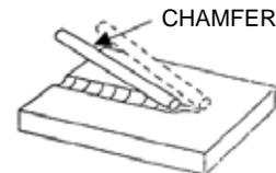
force of the GROOVE ROD arc removes the molten metal, by pushing it out in front of the groove, with a forward and backward motion. Where possible, the work should be inclined so that the molten metal can run free under the force of gravity.
