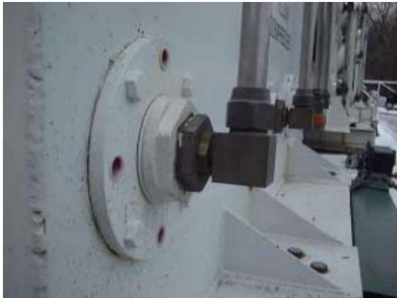
Figure 1—Pressure relief device assembly for the front end of a tube trailer
