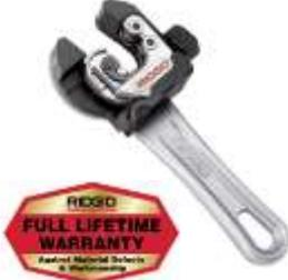
Allows for fine indexing - of the cutter - to operate in tight spaces. The new ratchet handle allows more flexibility and mobility while keeping the AUTOFEED features of the standard model #118 Cutter, which is designed to cut hard and soft copper, aluminum and brass from 1/4" through 1-1/8" OD. Comes with a spare E-3469 Cutter Wheel (stored in the knob).
