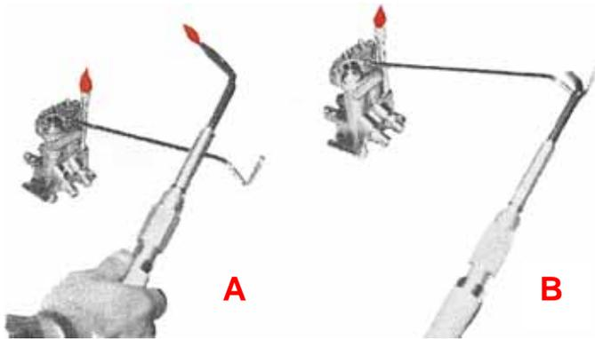
**A** shows the ignited torch about to be hung on the lever rod of the Gasaver.
