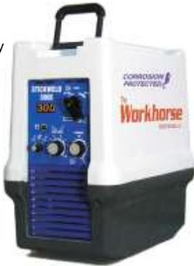
**The Workhorse 300ST** is a rugged DC (Arc Start) TIG and Stick welder primarily designed for TIG welding (GTAW) using time-proven SCR-inverter type technology. The single pulse capacitor arc starter does not produce high frequency radio noise, which can interfere with cell phones and other communication systems. Automatic Pre & Post flow gas control is standard.
