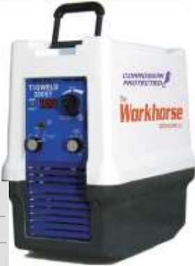
**The Workhorse 300MS** is an industrial DC power source that can be used for MIG short arc (with puddle control) and spray transfer, easy strike STICK welding. The 14-pin remote connector accepts a wide variety of wire feeders and spool guns (with 24VAC, 42VAC, and 115VAC power).
