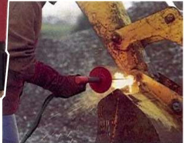
The SLICE torch cut through a frozen pin on this backhoe in less than a minute
