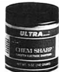
**Procedure:** Extend tungsten end out about 1" beyond cup. Short out tungsten against ground clamp or workpiece until end glows cherry red approximately 3/8" from tip. Quickly immerse the heated tip approximately 1/4" deep into the CHEM SHARP repeatedly until the point is formed.
