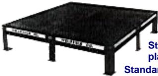
**Round Counter Sunk Holes Keep the Entire Work Surface Clear of Bolt Heads.** Heads of the mounting bolts are recessed below the work surface. Bolting the platen to the stand eliminates any unwanted moving or shifting while removing the workpieces.
