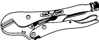
Designed for the refrigeration industry. Pinches off and locks on copper tubing instantly. Leaves both hands free. Ideal for emergencies - no shut-off valves needed. Easy release trigger.
