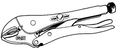
Two sizes - 10" and 7". Both have curved jaws for better contact on bolt heads, nuts and round work. Simply turn the micro-adjusting screw to set jaws for proper size and pressure, or for pliers action.
