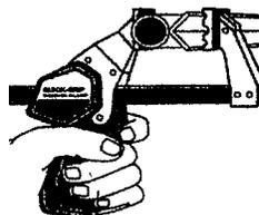
Horizontal and vertical grooves on jaw surface allow easy clamping of round stock.
