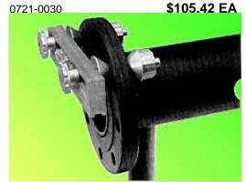
If adjacent top or bottom holes cannot be used, two-holing can be achieved using side bolt holes. In this instance, the DSL dial is set at 90 degrees and the flange is rotated until the bubble is centered.
