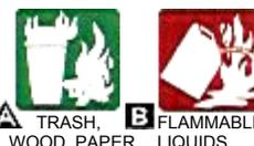
While foams are primarily desired protection for class "B" flammable liquid hazards, the wetting and cooling characteristics of an AR-AFFF foam solution also make them effective on class "A" common combustible types fires.
